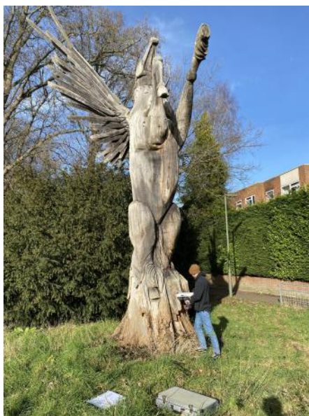
Decay testing of Pegasus using a resistograph machine.
